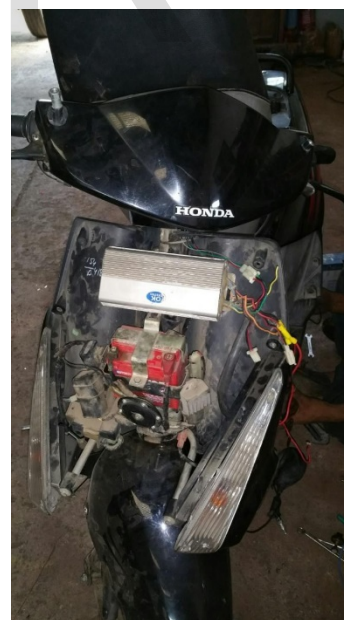
Fig. 4. Front view of the Hybrid Two-wheeler showing the assembly of the controller.
